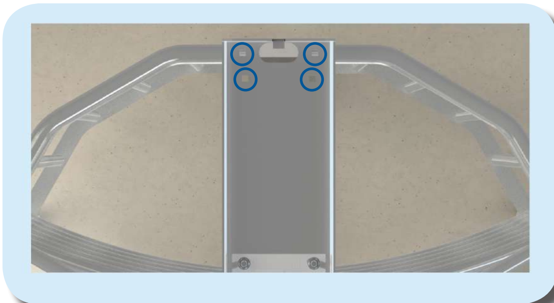
Fig-5.20 Correctly Fitting Channel to Frame Fixings
