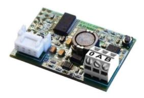
Wi-Fi expansion card for U-Link BFT products that allows the user and the installer to remotely control (via Wi-Fi, 4G connection or TCP/IP) the gate motor from smartphones and laptops.
