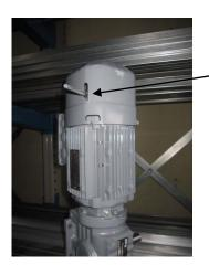
3. Insert and screw into end cap of induction motor, located within the small opening
